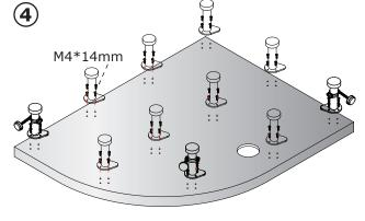
Screw the feet in position with the screws provided. Ensure that the feet that have panel fixing rod attached, are placed around the curved edge where the panels will meet.
