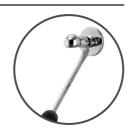
Connect the shower handset to the conical end of the hose, ensuring the hose washer is fitted and place in the handset holder. THE FRICTION OF THE HANDSET HOLDER IS FACTORY SET AND SHOULD NOT BE ADJUSTED.
