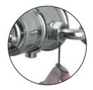
Tighten the inlet compression unions sufficiently to ensure a watertight seal. Push the cover plates over the unions flush to the wall surface.
