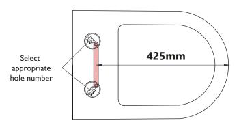
3 Once the 425mm dimension shown above is met and the template is parallel to the back edge, insert the bolts then tighten using a screw
