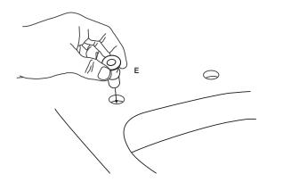
If difficult to push in, lubricate the rubber insert with water.
