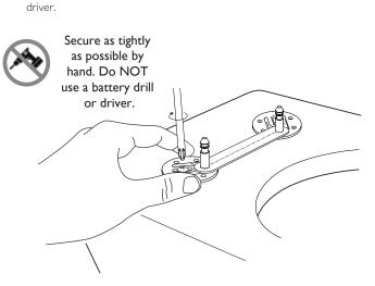
4 Remeasure the distance, making sure the 425mm dimension is met and remove the template and add the cover cap.
