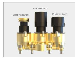
For push button models. Screw the black extension caps onto the headworks. (Use the shorter ones for 60-70mm installation depths OR the longer ones for 70-80mm installation depths.)
