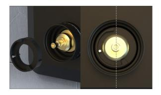
5. Fit the white spacer ring and flow control dial before placing the temperature override cam onto the shaft. Ensuring it is in the correct orientation(vertical – as shown).
