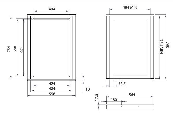
Diagrams not to scale All dimensions in mm Tolerance of +/-5mm
