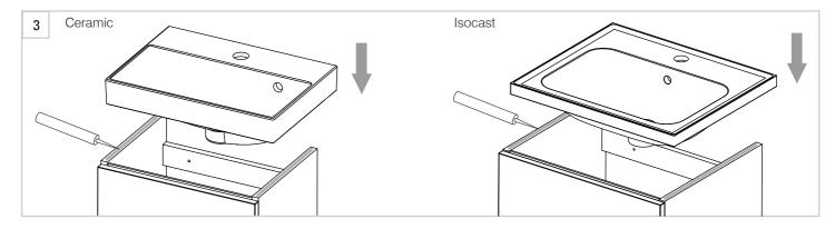
Finish by securing the basin to the washstand with a silicone sealant (not supplied).
