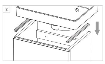
Apply the rubber extrusion to the side panels prior to applying silicone.
