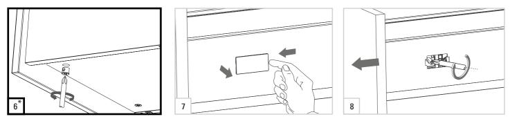
\*Release the cam bolt or unscrew the L-bracket on the bottom face of the drawer before releasing the drawer fascia.
