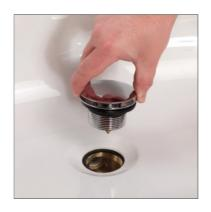
4. Ensuring the rubber washer is correctly aligned, pass the bath waste clicker through the bath and secure to the waste body assembly. Connect the bath waste to a suitable trap (not supplied).
