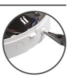
Screw in the two upper fixing screws leaving the heads projecting about 10mm from the wall surface. Feed the working end of the low voltage cable through the entry point in the back plate. Locate the back plate in position on the projecting screw heads. Ease the back plate downwards and engage the screws in the slots. Fix the lower fix screw and tighten the upper fixing screws.
