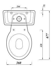
All dimensions are in milimetres unless otherwise stated. The information contained on this page was correct at date of issue. Fitting dimensions are provided as a quide only. Some variation may occur due to manufacturing tolerances. We pursue a policy of continuing improvement in design and performance of our products and so reserve the right to change specifications without prior notice.
