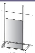
1 x Glass panel 1 x Floor to ceiling post Tray must be at least 100mm up to door dimension
