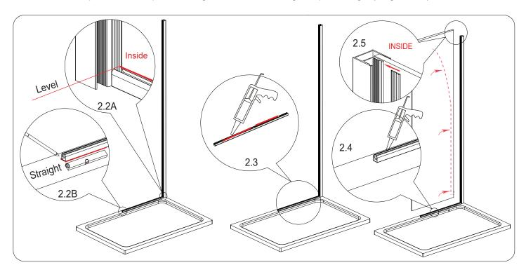
**Step 2.2** Remove the fixed panel then replace the bottom strip (Part 11) onto the tray, ensure the bottom strip groove is level to the wall profile groove on the inside face (Diagram 2.2A). Mark the line on the tray for the bottom strip position once you have ensured it is straight. (Diagram 2.2B)
