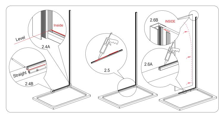
**Step 2.4** Remove the fixed panel then replace the bottom strip (Part 11) onto the tray, ensure the bottom strip groove is level to the wall profile groove on the inside face (Diagram 2.4A). Mark the line on the tray for the bottom strip position once you have ensured it is straight. (Diagram 2.4B)
