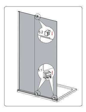
Step 5.1 Ensure the gasket has been placed inside the roller then fit it to the door panel from the bottom, roughly the roller should be about 50mm to the glass end. Ensure the soft head is attached on the grub screws then attach the roller together with the glass panel. (Diagram 5.1)
