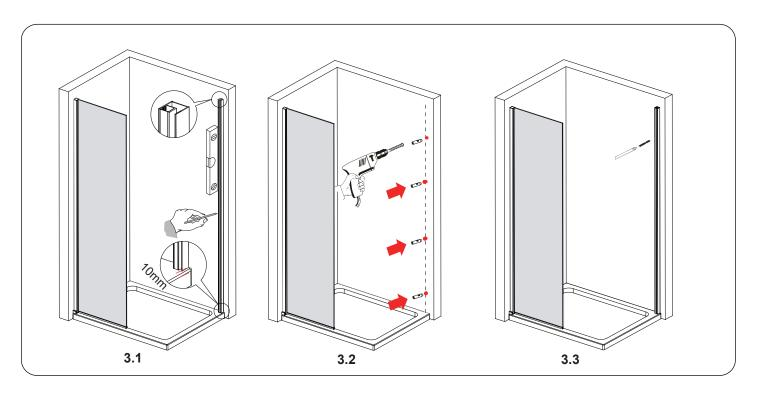
Step 3.1 Place the side panel Wall Profile (part 33) onto the tray,roughly 10mm away from the front edge of the end cap. Level the wall profile using a spirit level then mark the profile through the pre-drill holes on the wall profile (Diagram 3.1)
