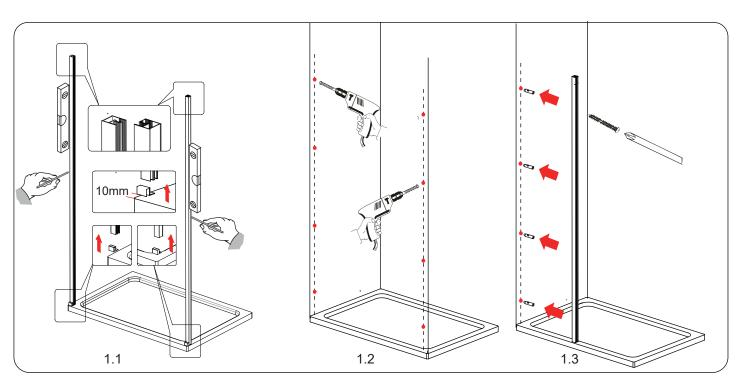
**Step 1.1** Fit the Bottom Rail End Cap L/R (Part 10) on the fixed panel wall profile (Part 2) and closing wall profile(Part 29) from the bottom. Place the wall profiles onto the tray,rough 10mm away from the front edge of the end cap. Level the wall profiles using a spirit level then mark the profile through the pre-drill holes on the wall profiles. (Diagram 1.1)
