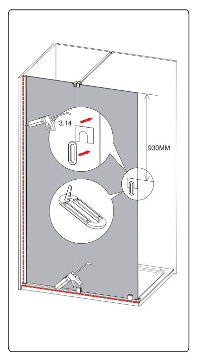
**Step 3.13** We do not recommend fitting the vertical seal (Part 7) onto the fixed panel as the overlap between the fixed panel and door panel will be sufficient to avoid any leaks. If you do decide to fit vertical seal please ensure you cut it as detailed in diagram 3.13. to avoid any obstruction to the handle or rollers.
