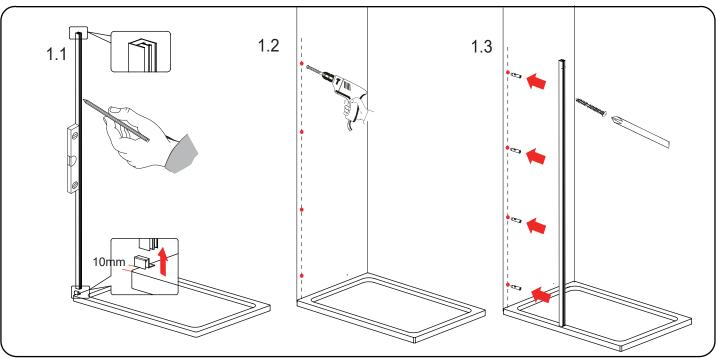
**Step 1.1** Fit the Bottom Rail End Cap L/R (Part 10) on the wall profile (Part 2) from the bottom. Place the Wall Profile onto the tray, roughly 10mm away from the front edge of the end cap. Level the Wall Profile using a spirit level then mark the profile through the pre-drill holes on the Wall Profile. (Diagram 1.1).
