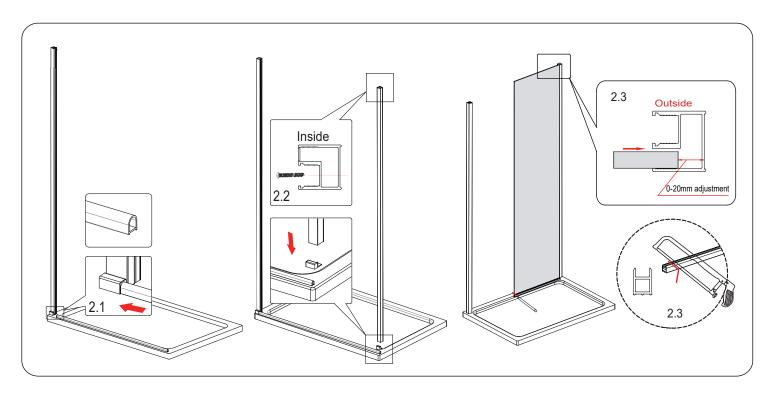
Step 2.1 Cut the bottom rail (part 12) to the required length then insert it into the end cap L(Part 10) fitted on the fixed panel wall pofile. (Diagram 2.1)
