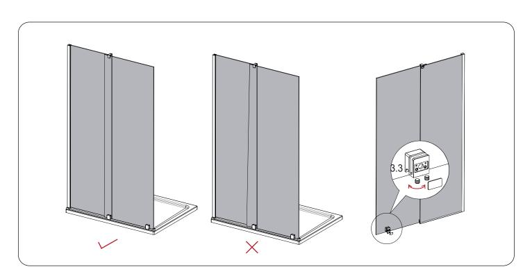
**Step 3.3** Check the door to make sure the door panel is level with the fixed panel. If not remove the door panel and loosen the fixing grub screws, then raise or drop the door panel by tightening or loosening the grub screws pre-fitted at the bottom of the roller. Once the door panel is in the perfect position fit the roller screws caps onto the roller. (Diagram 3.5)
