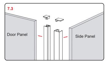
**Step 7.3** Take the 3M adhesive tape back away then drop the silicone sealant onto the groove of the magnet profiles, fit the magnet profile onto the door panel and side panel. Once this is done fit the top cap onto the magnet profile. (Diagram 7.3).
