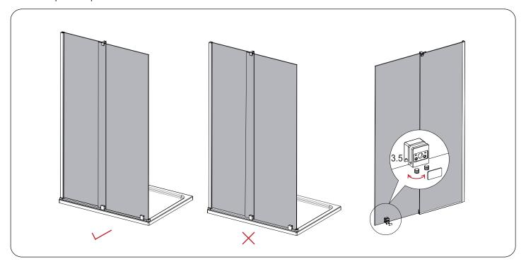
**Step 3.5** Check the door to make sure the door panel is level with the fixed panel. If not remove the door panel and loosen the fixing grub screws, then raise or drop the door panel by tighten or loosening the grub screws pre-fitted at the bottom of the roller. Once the door panel is in the perfect position fit the roller screws caps onto the roller. (Diagram 3.5)
