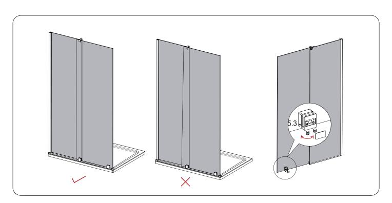
**Step 5.3** Check the door to make sure the door panel is level with the fixed panel. If not remove the door panel and loosen the fixing grub screws, then raise or drop the door panel by tighten or loosening the grub screws pre-fitted at the bottom of the roller. Once the door panel is in the perfect position fit the roller screws caps onto the roller. (Diagram 5.3)
