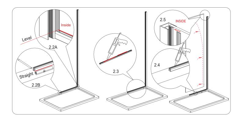
**Step 2.2** Remove the fixed panel then replace the bottom strip (Part 11) onto the tray, ensure the bottom strip groove is level to the wall profile groove on the inside face (Diagram 2.2A). Mark the line on the tray for the bottom strip position once you have ensured it is straight. (Diagram 2.2B)
