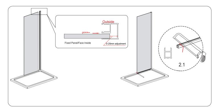
**Step 2.1** Carefully lift the fixed panel (Part 3) and insert into the wall Profile groove, it allows 0-20mm for the adjustment. Once the fixed panel is in required adjustment, place the bottom strip(Part 11) onto the tray and mark a line onto the profile. Cut the profile through the marked line to get required length. (Diagram 2.1)
