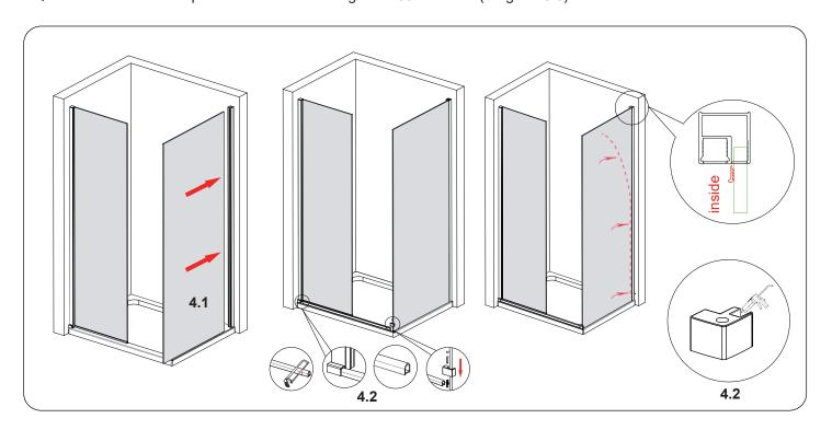
**Step 4.1** Carefully lift the Side Panel Glass (Part 34) onto the tray,insert it into the wall profile channel. It allows 20mm for the adjustment.(Diagram 4.1)
