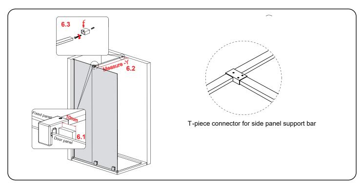
**Step 6.1** Ensure the glass clamp is in about 10mm away from the fixed panel edge(Diagram 6.1) then attach it onto the fixed panel using M10 x6 grub screw(Part 20)
