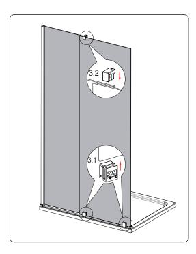
Step 3.1 Ensure the gasket has been placed inside the roller then fit it to the door panel from the bottom, roughly the roller should be about 50mm to the glass end. Ensure the soft head is attached on the grub screws then attach the roller together with the glass panel (Diagram 3.1).
