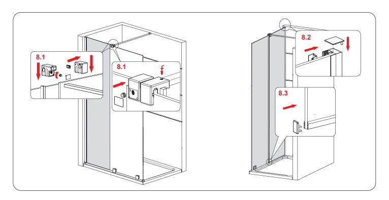
**Step 8.1** Fit a soft head (part 22) onto the roller stopper (part 25), then slide the door panel to ensure it touches the side panel glass, fit the roller stopper onto the door panel, ensure the soft head on the roller stopper touches the glass clamp then secure the roller stopper onto the door panel using M10x6 grub screw(Diagram 8.1)
