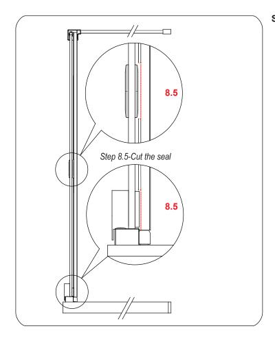
Step 8.5 We do not recommend fitting the vertical seal (Part 7 in the sliding wetroom carton) onto the fixed panel as the overlap between the fixed panel and door panel will be sufficient to avoid any leaks. If you do decide to fit the vertical seal please ensure you cut it as detailed in Diagram 9 to avoid any obstruction to the handle or rollers.
