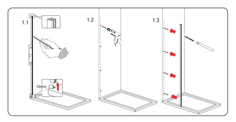
**Step 1.1** Fit the Bottom Rail End Cap L/R (Part 10) on the wall profile (Part 2) from the bottom. Place the Wall Profile onto the tray, roughly 10mm away from the front edge of the end cap. Level the Wall Profile using a spirit level then mark the profile through the pre-drill holes on the Wall Profile. (Diagram 1.1).
