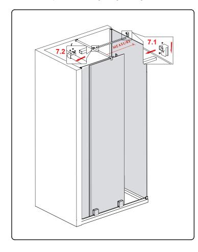
Step 7.1 Measure the support bar tube length then cut it to the required size, fit the Glass Clamp(Part 29) onto the side panel then secure it onto the side panel using a M10 grub screw(Diagram 7.1)
