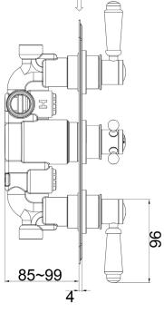
1. Temperature: pre-set 38°C with push button overide to 48°C 2. Automatic shut off in the event of hot or cold water supply failure
