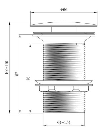
**Product Code:** Gunmetal Grey 167.PBBUSGM Fitting: G1-1<sup>1</sup>/<sub>4</sub>" BSP Male thread
