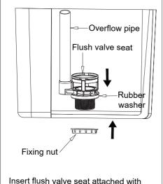
rubber washer into cistern flush hole. Then install and tighten with the fixing nut.
