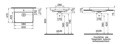
All drawings contain the necessary measurements which are subject to standard tolerances. For exact measurements, in particular for customized installation scenarios, it can only be taken from the finished ceramic product.
