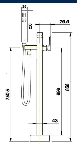
**Cartridge:** 35mm Ceramic disc cartridge
