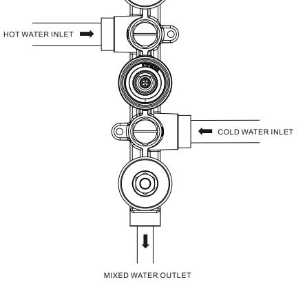
2.Connect the valve with the hot and cold water pipes (cold and hot water shall not be connected to the opposite, otherwise, it cannot be operated correctly), connect the mixed water outlets to the shower head, handset, or spray head, and check whether the joints are leaking.
