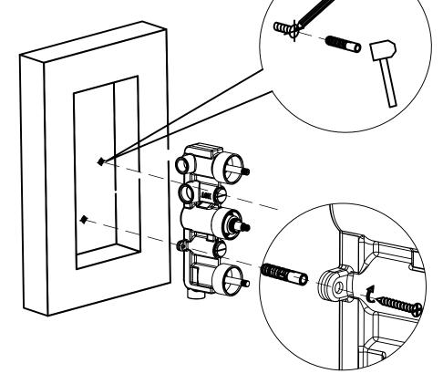
1.Determine the mounting position for the valve, refer to installation dimension drawings, reserve the recess in the wall in which to mount the valve, the depth of the recess should be min 72mm, max 82mm. Fix the valve with tapping screws and wall plugs.
