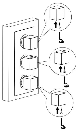
5. Tighten all the handle grub screws with Allen key.
