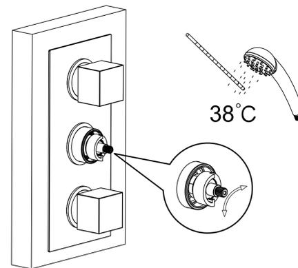
7. If there is a large deviation of the outlet water temperature from the default 38°C (deviation of  $\pm 2^\circ\text{C}$  is the normal range), remove the thermo handle, fine-tune the handle left and right to adjust the water temperature to  $38\pm 2^\circ\text{C}$ , and then reinstall the thermo handle.
