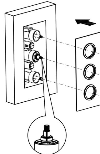
3. Check if the marking line of the thermostatic cartridge are aligned, and then put on the cover plate.
