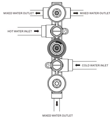
2. Connect the valve with the hot and cold water pipes (cold and hot water shall not be connected to the opposite, otherwise, it cannot be operated correctly), connect the mixed water outlets to the shower head, handset, or spray head, and check whether the joints are leaking.
