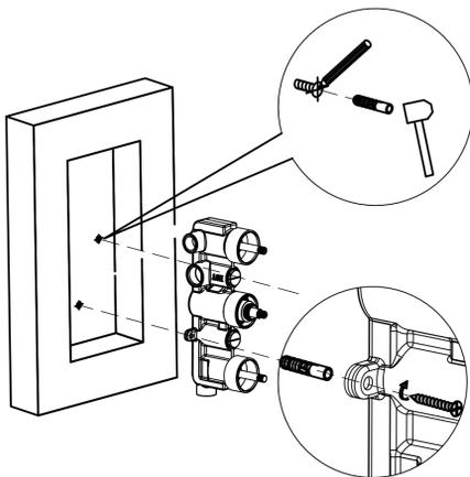
1. Determine the mounting position for the valve, refer to installation dimension drawings, reserve the recess in the wall in which to mount the valve, the depth of the recess should be min 72mm, max 82mm. Fix the valve with tapping screws and wall plugs.
