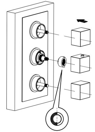
4. Install the thermo stop-ring, thermo handle, flow handle.
