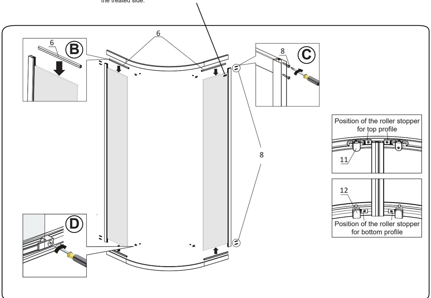
**E.1** Place the wall profiles onto the enclosure. Position the enclosure onto the tray. Ideally the enclosure should be positioned 10mm from the edge of the tray as shown. Centralize the enclosure onto the tray top rim and position vertically plumb using a spirit level.
