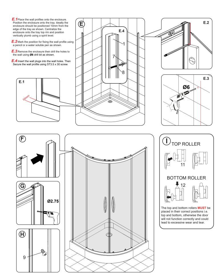
**G** Drill 3 equally spaced holes with a 2.75mm drill bit through the wall profiles and frame.
